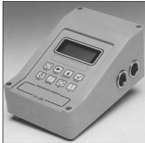
The TR200 loadmeter is a completely portable, precision instrument packaged in a small IP65 enclosure, for use with strain gauged loadcells.
