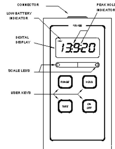
**The unit is supplied calibrated to a particular load cell. All user functions are available via the front keypad. Do not open the enclosure to make any adjustments.**
