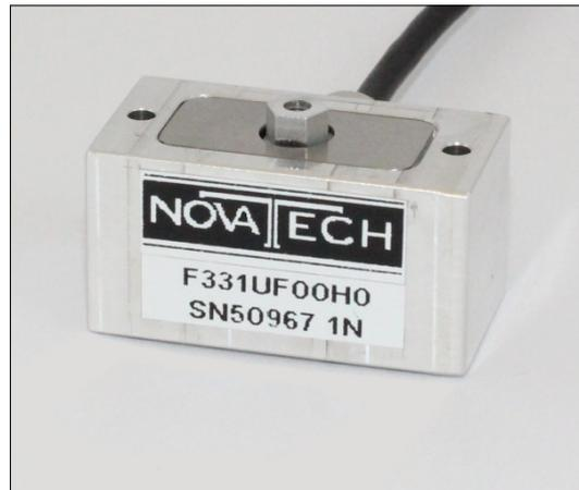
The F331 low range loadcell has been developed to meet a growing need for high resolution, low range force measurement with minimal translational deflection. The high stiffness of these loadcells, combined with their robust construction, lends themselves particularly well to dynamic and/or fatigue applications.
