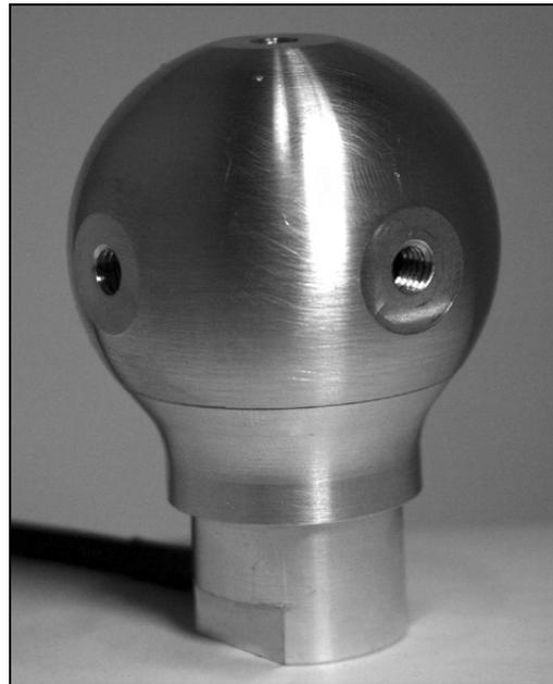
The F321 gear shift loadcell measures gear lever forces required to achieve gear selection. An ergonomically designed gear knob senses the force from a human hand or a mechanical actuator. The three axis force components are represented by three pure loadcell output signals. The gear shift loadcell is supplied calibrated and ready to use, no in-situ calibration or mathematical computation is required.
