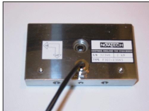
The F314 measures forces in two axes at 90°. Apart from error evaluations, each output is pure and requires no mathematical manipulation.
