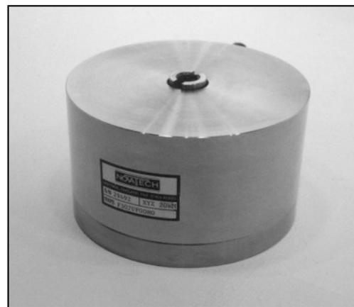
The F307 loadcell provides a bi-directional direct measurement of the X, Y and Z components resulting from a force vector. Apart from error evaluations, each output is pure and requires no mathematical manipulation.
