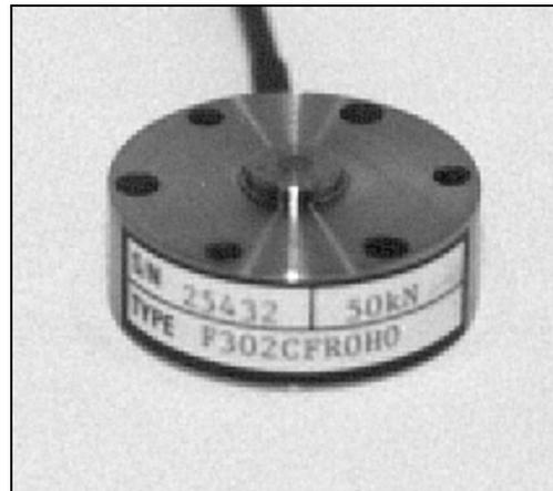
Geometry: Low profile axial loadcell for use in force measurements in compression.
