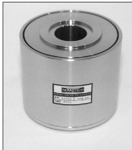
Geometry: Axial strain cylinder in weather sealed case, with raised end load bearing faces and hole right through. For use in compression or in fail-safe tensile applications.
