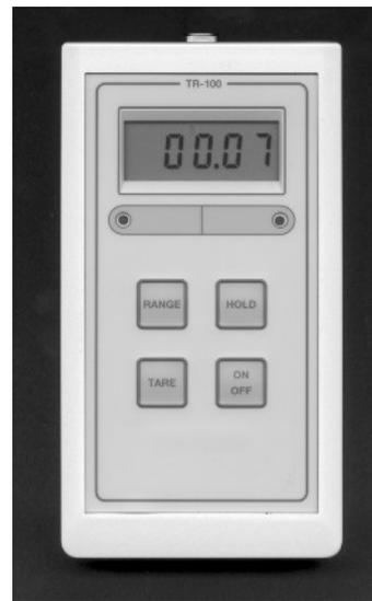
The TR100 loadmeter is a completely portable, precision instrument packaged in a small hand held IP65 enclosure, weighing only 260g.
