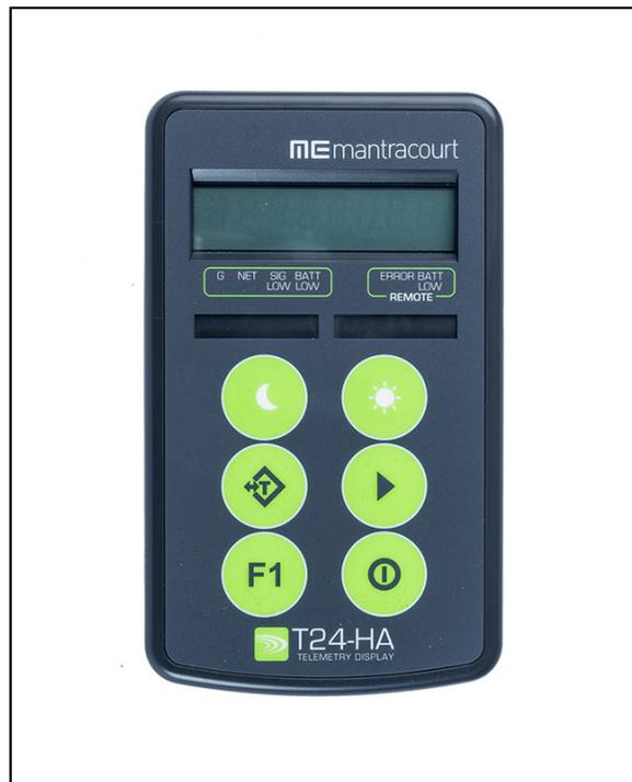
This wireless handheld display module provides an 8 digit LCD reading from up to twelve T24 loadcell data acquisition modules. The remote data acquisition modules can be 'powered on' and 'powered off' automatically as the T24-HA handheld is operated. Status indicators inform the user if the remote acquisition module has input integrity problems, low battery, low signal, over range or other error.
