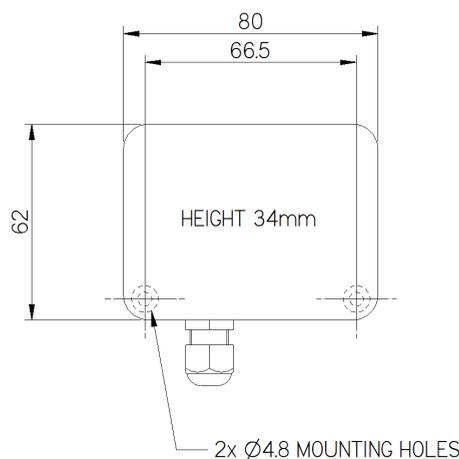
The unit is supplied with standard Binder 723 series cable mounted loadcell input socket mounted on an 80mm long cable.
