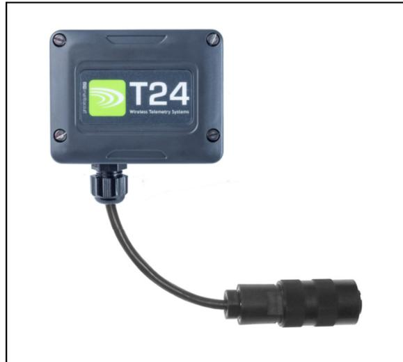
This miniature loadcell data acquisition unit provides high performance wireless measurement of loadcell outputs. Providing direct mV/V input and 5V bridge excitation for up to 4 load cells. Low power modes allow the module to 'power down' between transmissions or to 'power off' completely and can be controlled by other T24 products such as the handheld displays or a base station.
