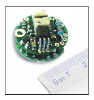
This miniature loadcell amplifier is designed for use with strain gauge loadcells. It has a bipolar  $\pm 10$ V output for use with bi-directional loadcells even though it is powered from a uni-polar supply.
