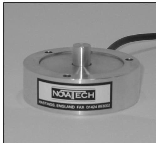
Geometry: Slender disc, with outer ring earth fixing and live inner boss usually shaft driven. This static torque transducer is used extensively in instrumentation and small electric motor test and calibration applications.
