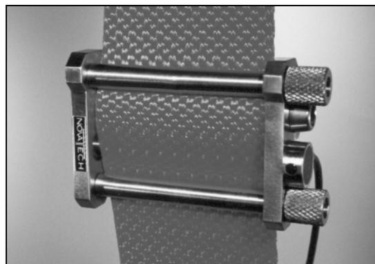
The F305 is a high performance loadcell for measuring seat belt tension forces. Its geometry was created by computer program to generate an optimal design with minimal mass, material usage, stress and deflection. The outer bars can easily be removed allowing fitting to a seat belt while it is anchored at both ends.
