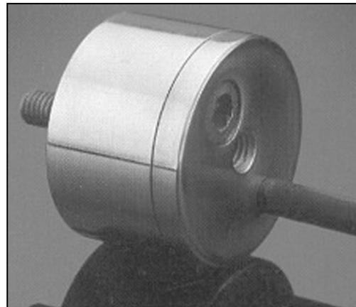
Geometry: Flexure strain assembly in cylindrical housing, open or weather sealed with end internal fixing. For universal use in tension and compression, with compensation for off axis load inputs.
