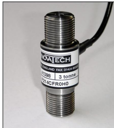
Geometry: Axial strain rod in weather sealed case, with external fixing threads. For use in tension or compression.
