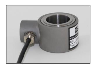
Geometry: Axial strain cylinder in a sealed case, with raised end load bearing faces and hole right through. For use in compression or in fail-safe tensile applications.
