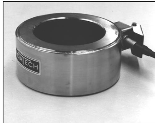
Geometry: Axial strain cylinder in a sealed case, with raised end load bearing faces and hole right through. For use in compression or in fail-safe tensile applications.
