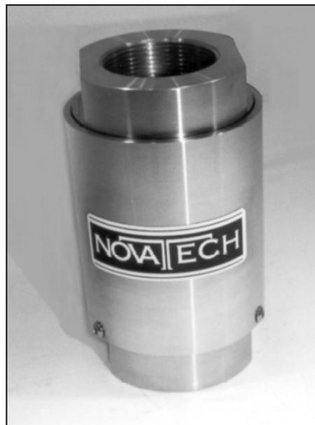
Geometry: Axial strain cylinder in a weather sealed stainless steel case, with end internal fixing threads. For use in tension and compression loaded in line with the axis. With bi-directional versions there is a small difference between the output signal for compression and tension. All standard bi-directional loadcells are calibrated in both modes and the output for each direction is stated on the test / calibration certificate.
