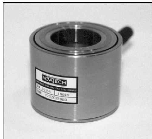
Geometry: Axial strain cylinder in weather sealed case, with raised end load bearing faces and hole right through. For use in compression or in fail-safe tensile applications.
